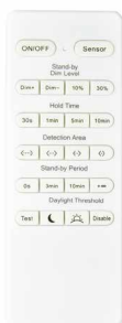
Remote for EVOX lamps microwave motion sensor Pilot do sterowania czujnikiem ruchu do lamp EVOX
